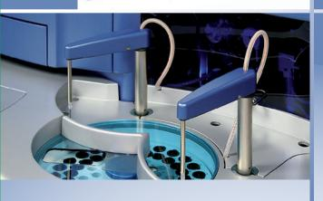
Besides Clinical Chemistry the analyzer can perform Turbidimetric tests, as well as Drugs of Abuse dosages. The I.S.E. module is available for indirect potentiometry K, Na, Cl,  $\rm CO_2$  or direct potentiometry K, Na, Cl, Li.
